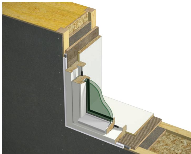
When the requirement of the window's sound insulation  $R_w+Ctr$  is lower than 32dB, it is recommended to insert the window and seal around it in accordance with Sintef construction details 523.701. (Standard installation).
