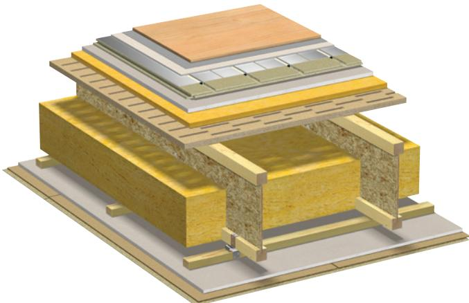
Fig. 6 Sound beam structure
