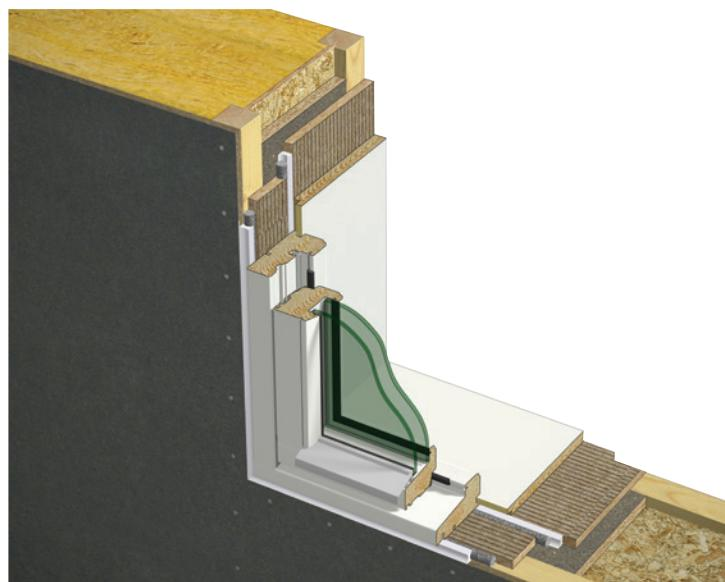
When the requirement of the window's sound insulation  $R_w+Ctr$  is greater than 32dB, it is recommended to insert the window and seal around it in accordance with Sintef construction details 533.109.
