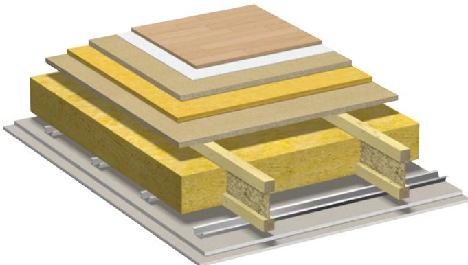
Fig. 7 Sound beam structure
